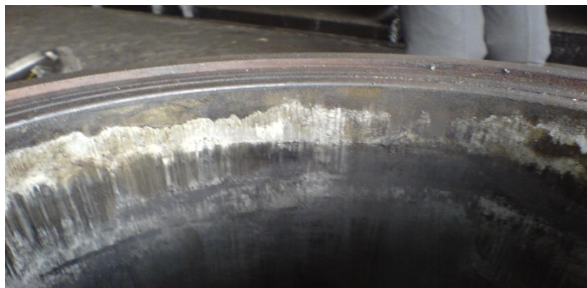
Fig.1.1 Effect of overheating of engine due to improper cooling system Engine works on the Diesel Cycle:
